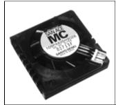
This compact fan measures just 44.5 mm sq.×10 mm thick, and is best suited for slim notebook personal computers that have little free space inside. It operates on 5 V DC, and is equipped with an ON/OFF control terminal.
